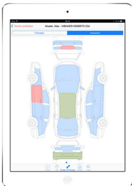
Based on the data stored in the customer field „Vehicle“ soft-pad will display the respective sketch of the vehicle, either a car, van or truck. In this sketch, you have the option to select individual vehicle segments such as the hood or the wind screen with their linked repair scopes from your repair catalog and save them directly within the appointment.
