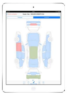
Based on the data stored in the customer field "Vehicle" soft-pad will display the respective sketch of the vehicle, either a car, van or truck. In this sketch, you have the option to select individual vehicle segments such as the hood or the wind screen with their linked repair scopes from your repair catalog and save them directly within the appointment.
